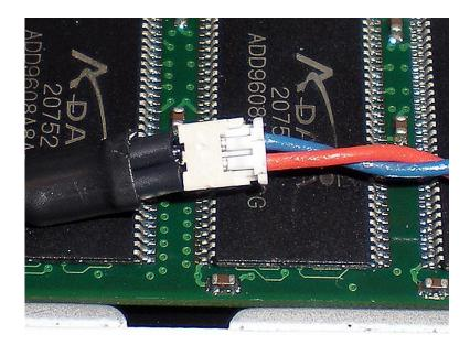
Tape the battery to the top of the memory card. Push the connector inside. Remount the lid with the screws.
