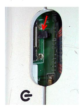
Cut the end of a Q-tip at an angle and use it to pull the actuator gently. Don't force the actuator when you don't see the blue light coming on immediately. It takes more than a second for the light to come on.
