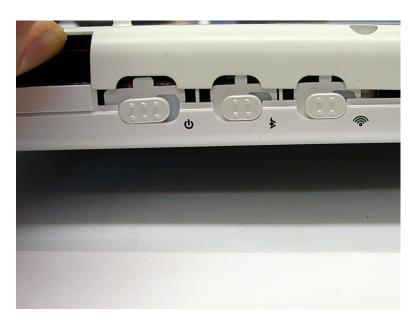
Try the on/off switch. If the cap was not snapped in properly, it will slide without activating the switch. If this is the case, repeat the process above.
