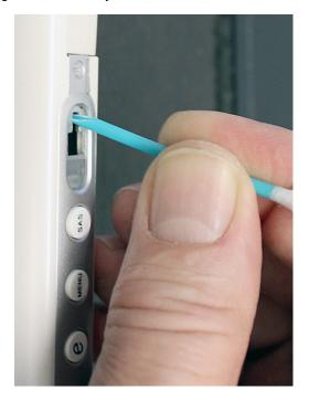
Slide in the new switch, aligned with the top position (left side on the picture), realign the other two caps to their bottom position (right on the picture), and snap together the shells.
