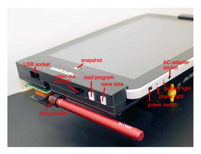
When installing the system, push the stylus, cap first, in the plastic loop at the bottom of the docking station, turning it clockwise to make it slide easier.
