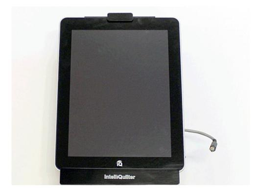
Plug in the power cable at the right edge of the tablet. **IMPORTANT NOTE: don't** forget to unplug the cable before removing the tablet from the docking station.
