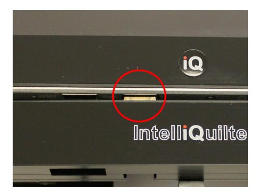
Push the top of the tablet toward the docking station and flip down the clamp.
