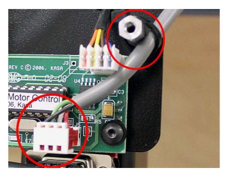
3. Remove the motor from the bracket by removing the two recessed bolts. Put back the bolts in the brackets, do not ship them with the motors.
